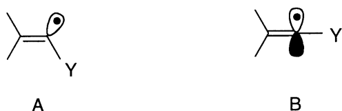
Fig. 1. Structures for \alpha -substituted vinyl radicals: A bent \sigma radical, B linear \pi radical
